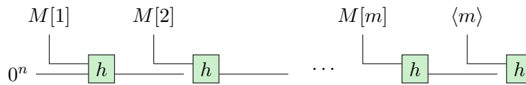
Figure 5.1: A visualization of the Merkle-Damgård transform, where h is any compression function.
